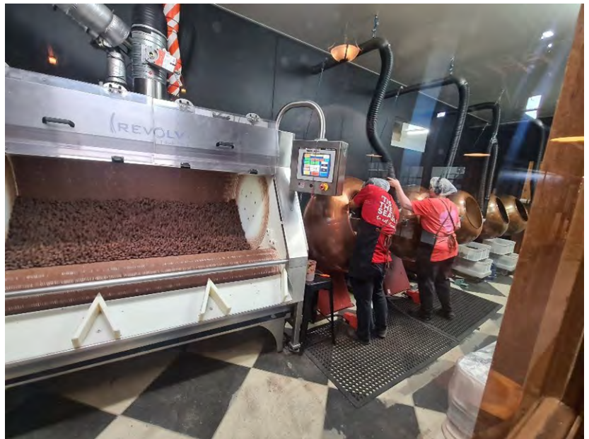
The chocolate coating machine for the heavier nuts like macadamias.
